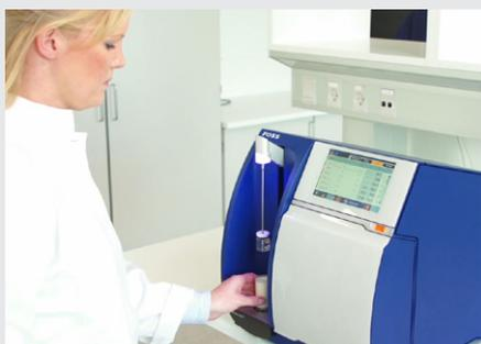
Place raw cold milk under the pipette, press start.
