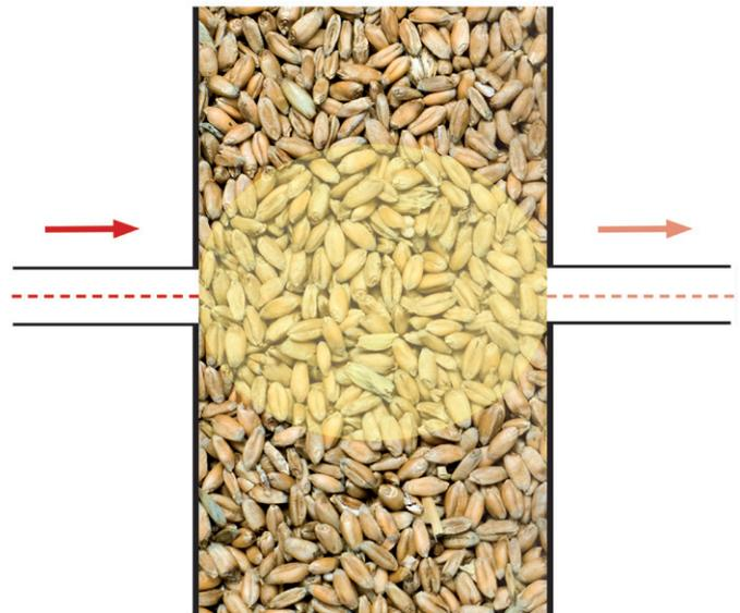
Every sub-sample is presented in the same way. In contrast, other solutions relying on gravity suffer from different compaction of each subsample which affects the information gathered.
