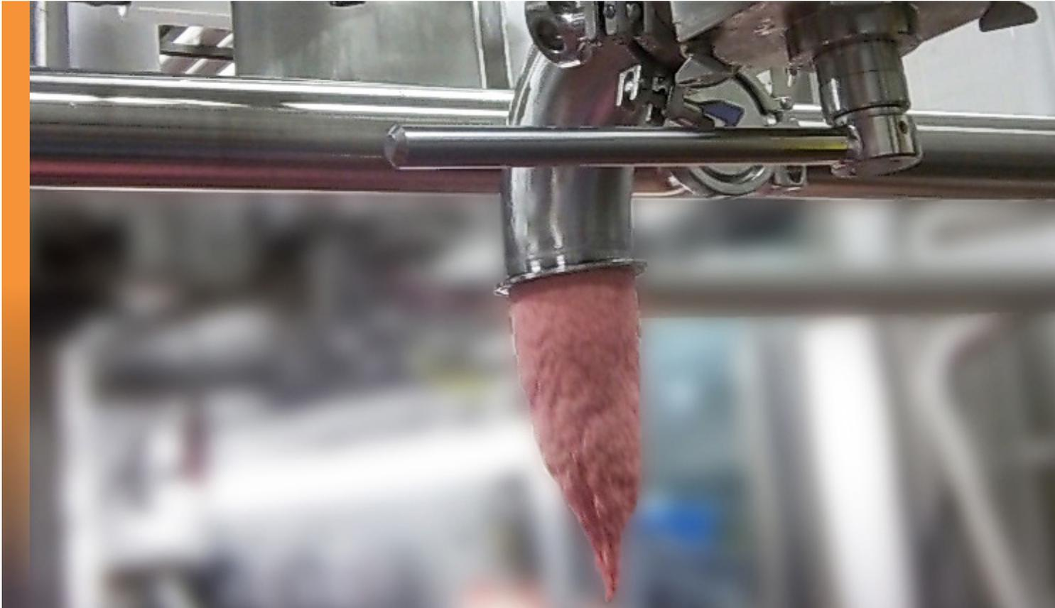
ProFoss™ solution for poultry MDM (Mechanical Deboned Meat) production provides a new way to control product quality while avoiding waste in the process. It consists of an analyser and a specially designed lateral transmission probe installed directly in the process pipe. The system performs analysis directly in the process line and feeds a continuous stream of analysis data to a computer/screen, giving you the possibility to monitor and control the production process.
