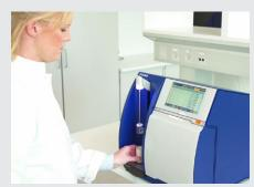
Place raw cold milk under the pipette, press start
