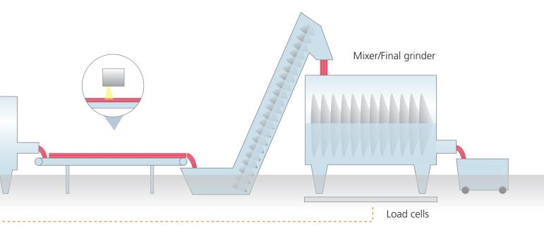
*Example of use: The ProFoss*<sup>TM</sup> solution can be installed to scan the meat above a conveyor. Several measurements are done during the processing of one batch. The results are displayed on a touch screen. The operator can follow the batch fat percentage and adjust if necessary.
